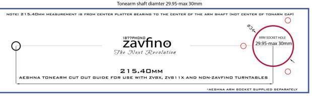
Adjust the collar with the hole for the tonearm with the distance to the center of the disc according the template (the distance have be 215,4 mm). The diameter of the hole for Aeshna Tonearms – 30 mm.
